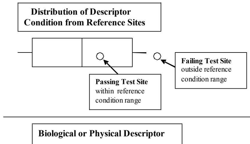
Figure 3. Comparing a feature (descriptor) of a site within a test stream to the reference condition derived from data describing conditions for several streams of the same morphological type as the test stream. (Adapted from Bailey et al. 2004).
