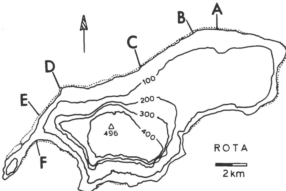
Figure 1. Rota Island, showing 100 m elevation contours (MSL datum), present reef margin (dotted lines), and sampling transect locations (lettered). Study area consists of the reef flat, where the Holocene limestone (HLS) is exposed, along the northern coastline and in the southwestern embayment (around Loc. F.). Scale is approximately 1:125,000.
